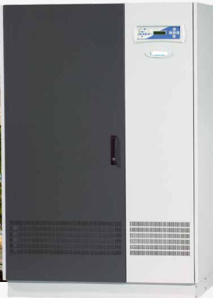
SERVOTEKNİK 300 Hi series UPS, PWM controlled, IGBT technology, microcontroller controlled, sinusoidal waveform, ONLINE topology and parallel configurable devices. Advanced communication system supports many communication protocols and brings remote control advantage of the UPS.
